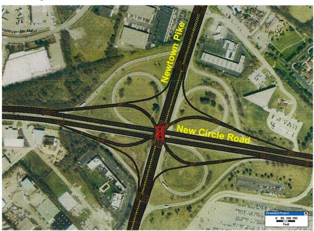
Figure 3: Single Point Urban Interchange (SPUI) at Newtown Pike
